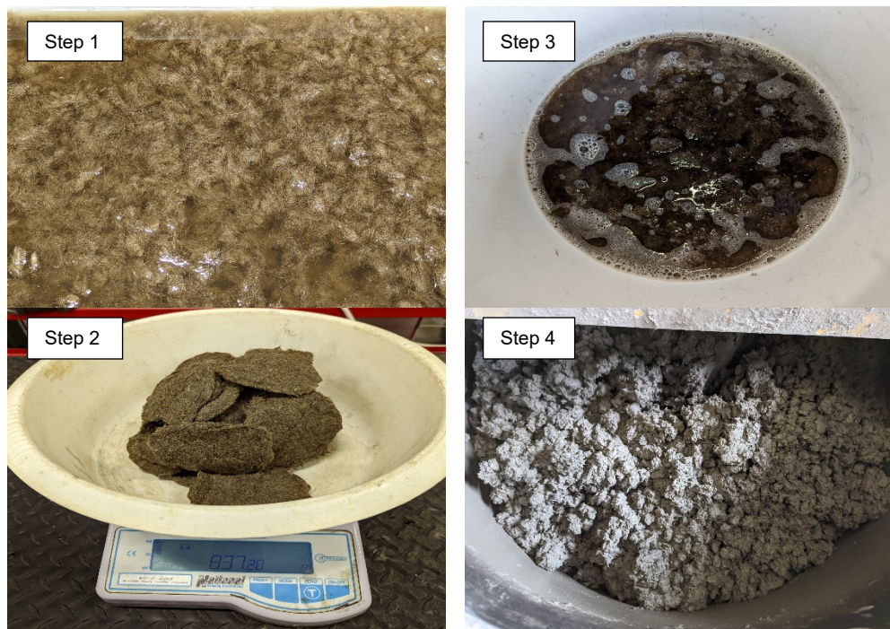
Figure 2. Batch mixing of hemp fibre - concrete composite
