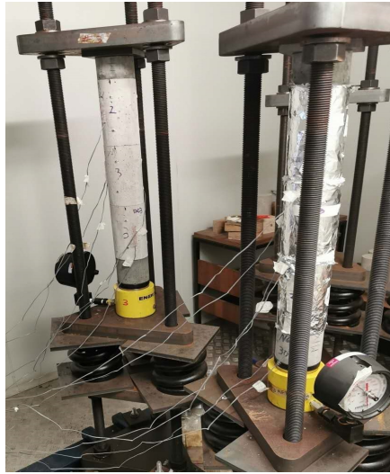
Figure 6. Creep testing of AABC (unsealed specimen left, sealed specimen right)
